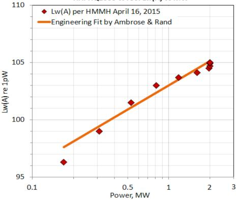
Good Engineering Fit: Lw(A) = 7log(MW) + 103, dB(A) re 1pW Accuracy: +/- 0.6 dB, 300 to 2000 KW
